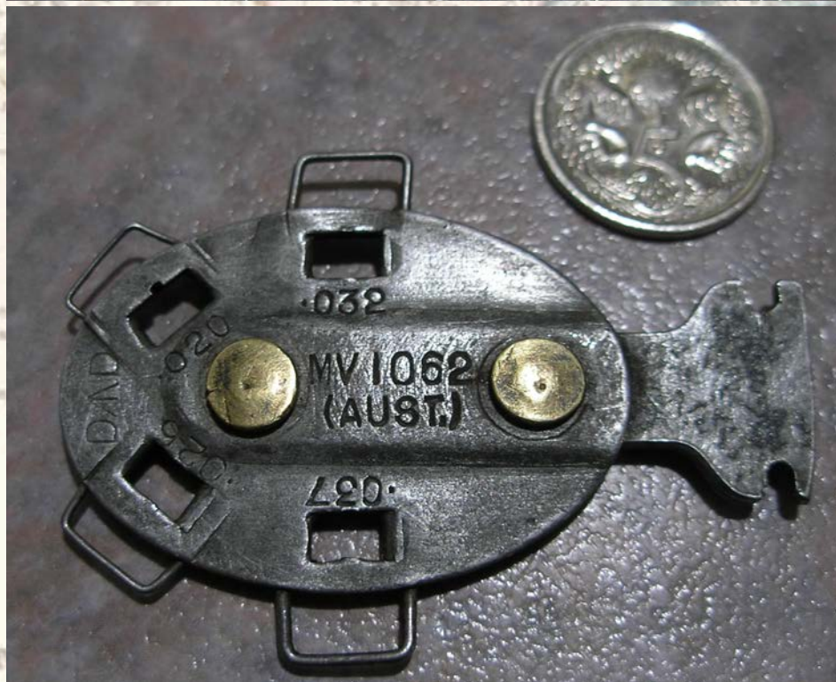
An interesting item used by a local member while serving in Vietnam. It is a tool for checking and setting the gap on spark plugs. Nice Australian markings.
